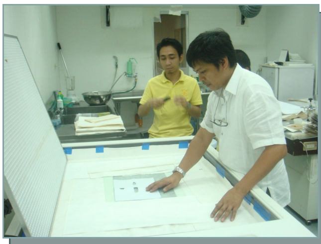
Mr. Rod Enano, restorer at the Roberto M. Lopez Conservation Center Laboratory, as he demonstrates how a leaf casting machine works.
