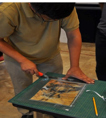
Encapsulation of a single sheet photo
